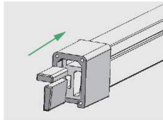
Stuff the plug into the holes corresponding to the led strip
