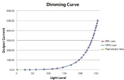
Note: Test data under 500mA gear
