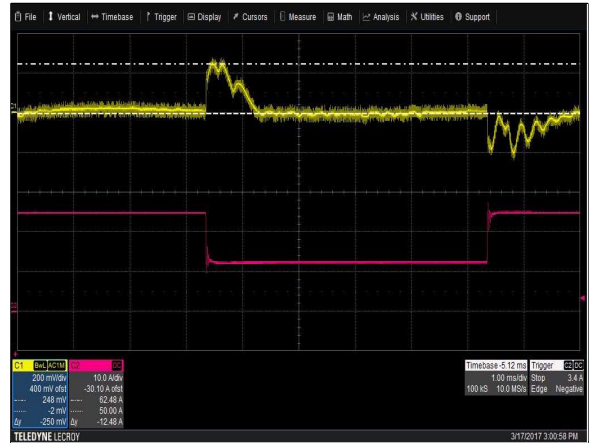
Figure 8: LCM300L Transient Response - V_O Deviation 100% to 50% load change 1A/uS slew rate V_{in} = 230V_{ac} Ch 1: V_O Ch 2: I_O
