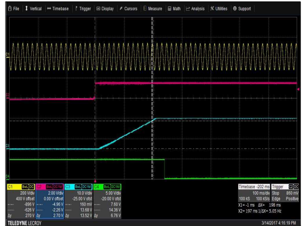
Figure 13: LCM300N Turn-on delay via INH_EN Vin = 90Vac Load: I O = 20A (15V), I SB = 2A (5V) Ch 1: AC Mains Ch 2: V SB Ch 3: V O Ch 4: G_DCOK_C
