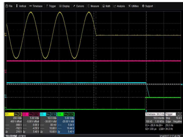
Figure 4: LCM300L Hold-up Time Vin = 264Vac / 60Hz / 0° Load: I O = 25A (12V), I SB = 2A (5V) Ch 1: AC Mains Ch 2: V SB Ch 3: V O Ch 4: G_DCOK_C
