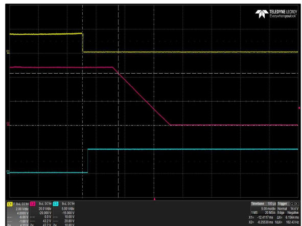
Figure 50: LCM300W Turn Off Characteristic via INH_EN Load: Io = 6.3A (48V), I SB = 2A (5V) Ch 1: INH_EN Ch 2: Vo Ch 3: G_DCOK_C
