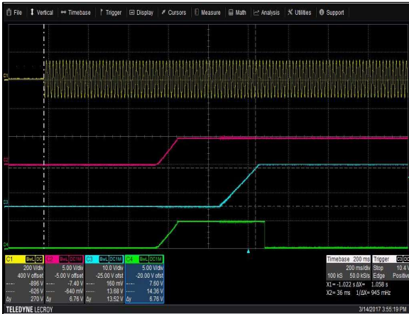
Figure 12: LCM300N Turn-on delay via AC mains Vin = 90Vac Load: I O = 20A (15V), I SB = 2A (5V) Ch 1: AC Mains Ch 2: V SB Ch 3: V O Ch 4: G_DCOK_C
