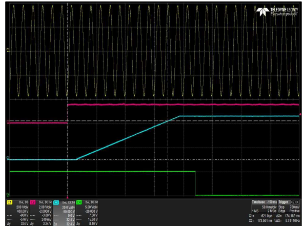
Figure 35: LCM300U Turn-on delay via INH\_EN V_{in} = 90Vac Load: I_o = 8.4A (36V), I_{SB} = 2A (5V) Ch 1: AC Mains Ch 2: V_{SB} Ch 3: V_o Ch 4: G_{DCOK\_C}
