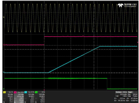
Figure 46: LCM300W Turn-on delay via INH_EN Vin = 90Vac Load: Io = 6.3A (48V), I SB = 2A (5V) Ch 1: AC Mains Ch 2: V SB Ch 3: Vo Ch 4: G_DCOK_C
