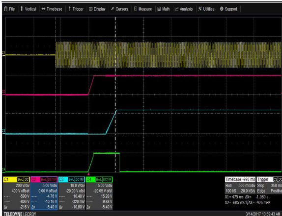
Figure 1: LCM300L Turn-on delay via AC mains Vin = 90Vac Load: I O = 25A (12V), I SB = 2A (5V) Ch 1: AC Mains Ch 2: V SB Ch 3: V O Ch 4: G_DCOK_C
