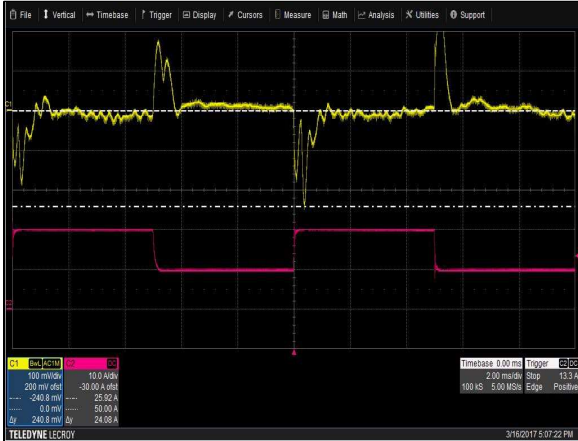
Figure 18: LCM300N Transient Response - Vo Deviation 50% to 100% load change 1A/uS slew rate Vin = 230Vac Ch 1: Vo Ch 2: Io
