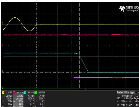
Figure 36: LCM300U Hold-up Time V_{in} = 90Vac / 47Hz / 0^\circ Load: I_o = 8.4A (36V), I_{SB} = 2A (5V) Ch 1: AC Mains Ch 2: V_{SB} Ch 3: V_o Ch 4: G_{DCOK\_C}
