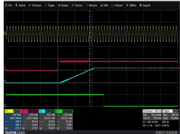
Figure 2: LCM300L Turn-on delay via INH_EN Vin = 90Vac Load: I O = 25A (12V), I SB = 2A (5V) Ch 1: AC Mains Ch 2: V SB Ch 3: V O Ch 4: G_DCOK_C
