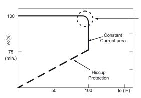
Typical LED power supply I-V curve
